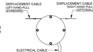
• Cable Pull - Series 150, 173, 174, 175, and 180 products provide a choice of either left-hand or right-hand displacement cable pull that provides increased mounting flexibility.
