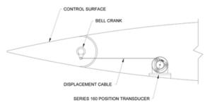
By locating the position transducers on both the flight control surfaces and cockpit controls, actuation delay, non-proportional control, and pilot-induced oscillations may be monitored.
