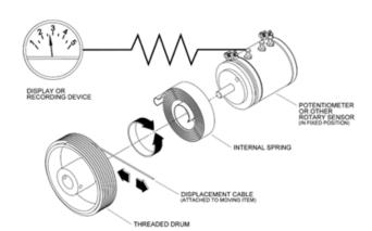
Figure 1.0: How a Position Transducer Works
