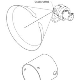
• Potentiometer Cover (part number 160060) - Protects the potentiometer on Series 16X products in adverse environments.
