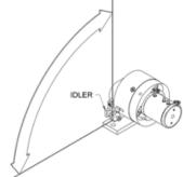
• Pulley - An Idler or pulley can be used to remotely position the transducer in high-temperature areas as well as to allow measurement through conduits and similar inaccessible areas.
