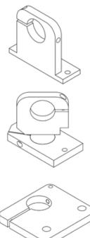
**Big Foot Base (part number 160015-13 or 160015-15)** - Similar to the standard base but with a wider mounting platform for quicker mounting.
